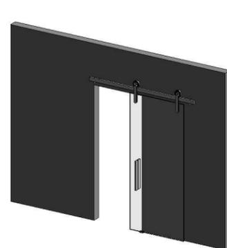
Solstice Sliding Door Single Solid Wall Installation
