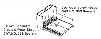
Sill to Subsill, End Dams, Screw Heads and Threshold to Door Frame Sealing.
