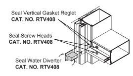
Small Joints, End Joints and Buttered Surfaces, Water Diverters and Reglet Fills.
