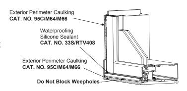
Perimeter Seals, Expansion Joints, Sill and Threshold Beds, Concrete, Wood and Steel Openings.
