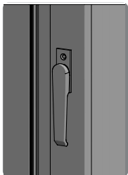
Catch Handle faces down when locked.
