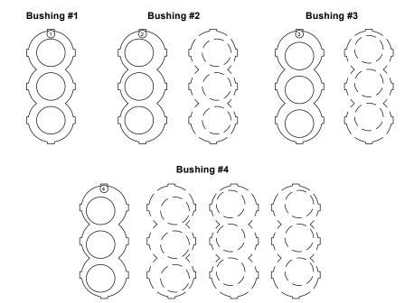
Use Bushing #4 when the "Hole Centers" and the 4 1/8" dimension from door's edge are both off 1/16" in either direction.
