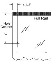
Use Bushing #1 when the "Hole Centers" dimension is correct and the 4 1/8" dimension from door's edge is accurate.
