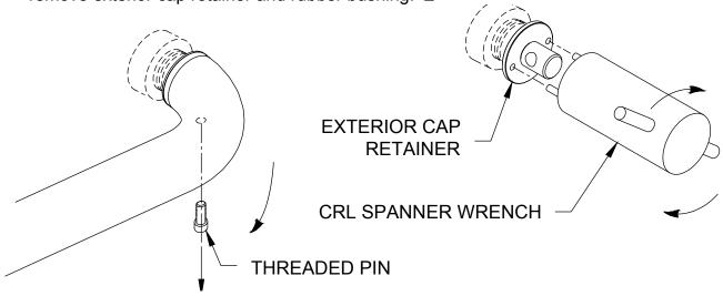
4. Unscrew the retainer cap holding the exterior horizontal handle to the plywood, being careful that the handle does not fall from the backside of the plywood.
