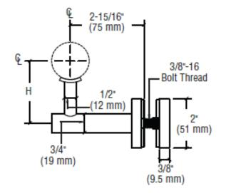
**GRAB RAIL BRACKET – HR3E Malibu Series** MOUNTED TO 1/2" GLASS PANEL Loading 200 lb concentrated load or 50 plf distributed load Grab rail bracket – 3/4" Dia. 316 Stainless steel bar threaded to the mounting plate.
