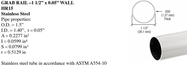
Stanless steel tube in accordance with AS1M A554-10 Rail Service Loading: Brushed stainless steel,  $F_y \ge 45$  ksi,  $F_u \ge 91$  ksi  $F_{cr} = \pi^2 k E_o / [12(1-\mu^2)(w/t)^2] = 4^* \pi^2 27,000 ksi / [12(1-0.3^2)(0.70/0.05)^2] = 124.5 ksi$  $\phi M_n = 0.9^* 1.25^* S^* F_y = 0.9^* 1.25^* 0.0799^* 45$  ksi  $\phi M_n = 4,045^{"\#}$  $M_1 = \phi M_n / 1.6 = 2,528^{"\#} = 210.67^{"\#}$
