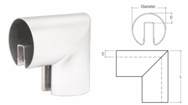
When the 6063-T6 aluminum alloy is welded the tempering is lost within the area of the weld affected zone reducing the allowable stress in the tubes to 5.5 ksi within 1" of the weld. This reduces bending strength to 30% of the bending strength for the unaffected cap rail.
