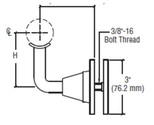
**GRAB RAIL BRACKET – HR2E Malibu Series** MOUNTED TO 1/2" GLASS PANEL Loading 200 lb concentrated load or 50 plf distributed load Grab rail bracket – 3/4" Dia. 316 Stainless steel bar attached to mount with 3/8" threaded rod. Bracket strength will be determined by couple between threaded rod in tension and compression in 3/4" bar edge.
