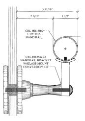
**GRAB RAIL BRACKET – HR2D Newport Series** MOUNTED TO 1/2" GLASS PANEL Loading 200 lb concentrated load or 50 plf distributed load
