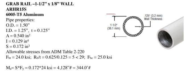
Allowable Span: Check based on simple span and cantilevered section.
