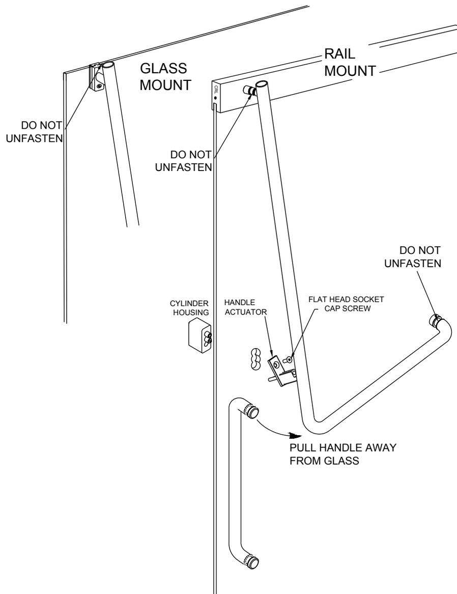
1. Hold on to exterior cylinder housing.
