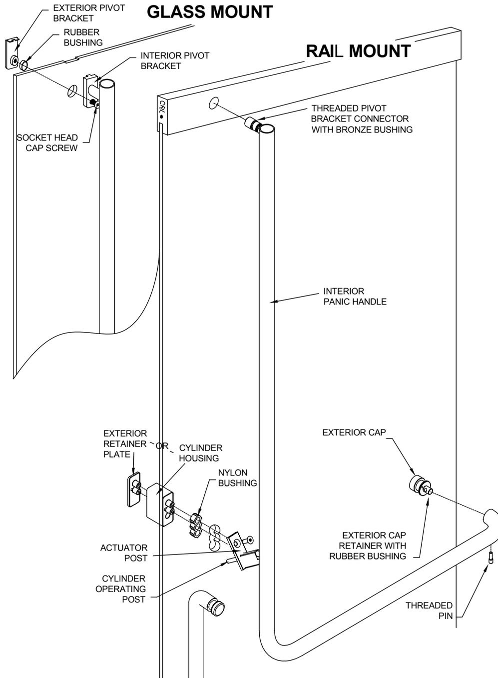
4. **RAIL MOUNT HANDLE:** Tighten the threaded pivot bracket connector to the adapter block at the top of the door.
