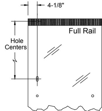
Use Bushing #1 when the "Hole Centers" dimension is correct and the 4 1/8" dimension from door's edge is accurate.
