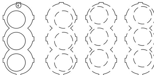
Use Bushing #4 when the "Hole Centers" and the 4 1/8" dimension from door's edge are both off 1/16" in either direction.
