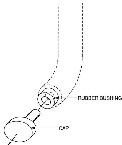
Apply **THREADLOCKER** to all fasteners used to mount handle on doors.
