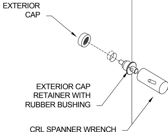
Apply **THREADLOCKER** to all fasteners used to mount handle on doors.
