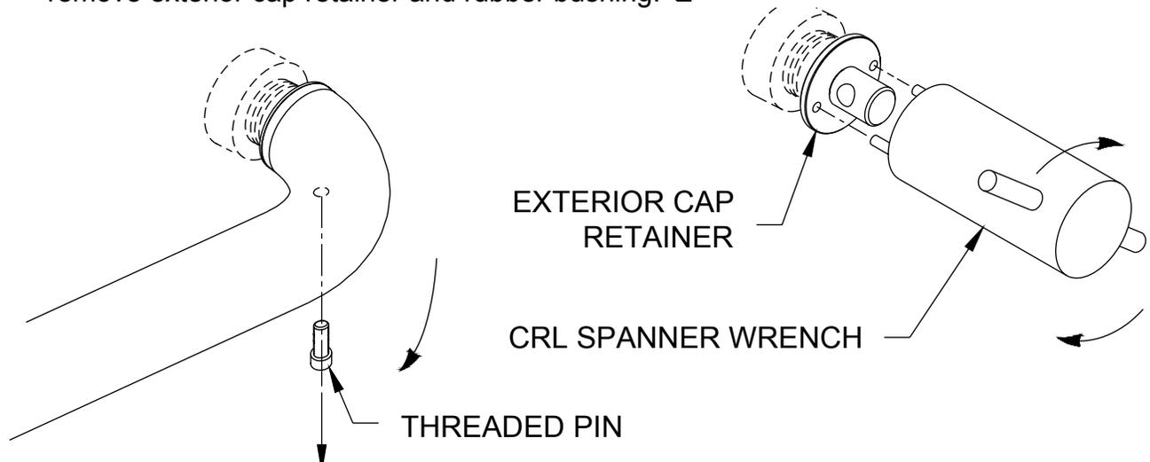
4. Unscrew the retainer cap holding the exterior horizontal handle to the plywood, being careful that the handle does not fall from the backside of the plywood. Remove rubber bushing for re-use during installation to the door. ➡
