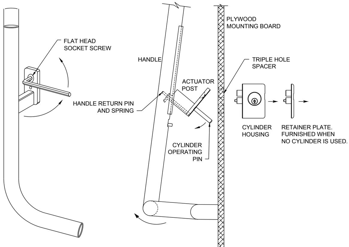
2. FOR RAIL MOUNT HANDLE. Rotate round connector pivot fitting counter clockwise and remove from Adapter Block. Note: Use pliers and rubber strip (to protect finish) for removal of round connector. ➔
