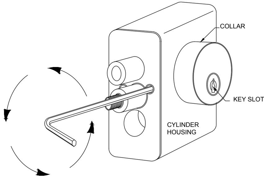
5. Remove old cylinder and check to see if tailpiece matches new cylinder tail piece. Also the length of the new cylinder must be the same as the old one. A cylinder of any other length will require a new length collar. Wind in new cylinder until it stops inside the collar ring. Key slot should be on bottom of cylinder nearest the floor.
