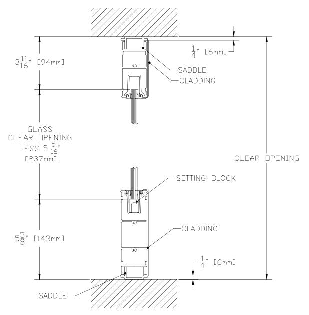
4" SQUARE SIDELITE RAIL WITH 1/4" SADDLE TOP 6" SQUARE SIDELITE RAIL WITH 1/4" SADDLE AND SETTING BLOCK BOTTOM CLAD OR NON-CLAD
