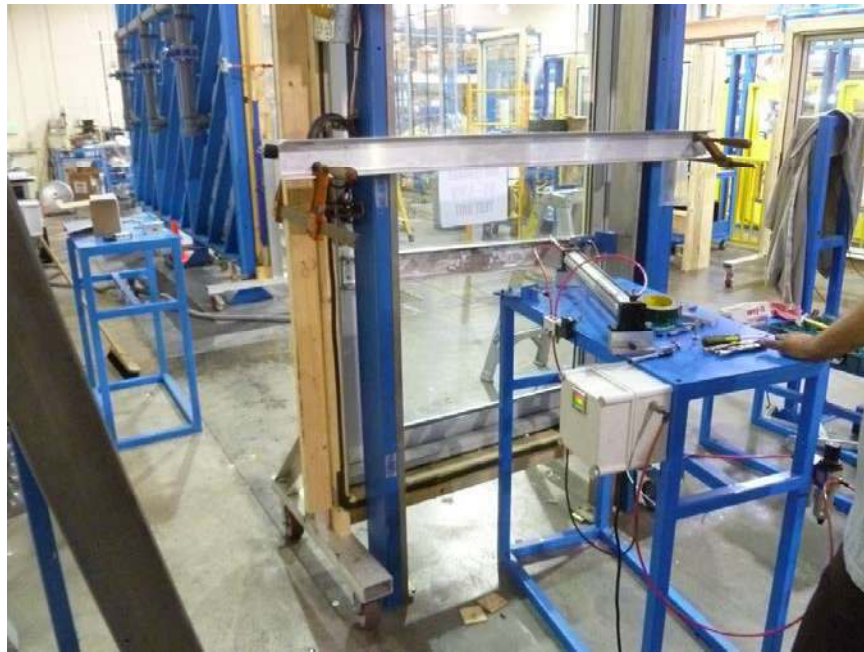
Photo No. 1 Door Cycling Set-up – Interior
