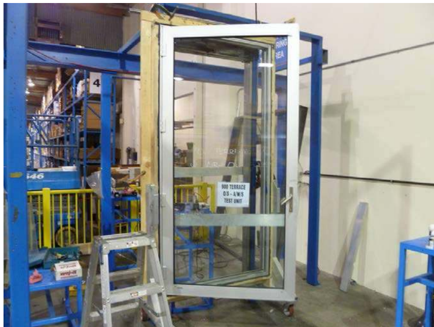
Photo No. 2 Door Cycling Set-up – Exterior
