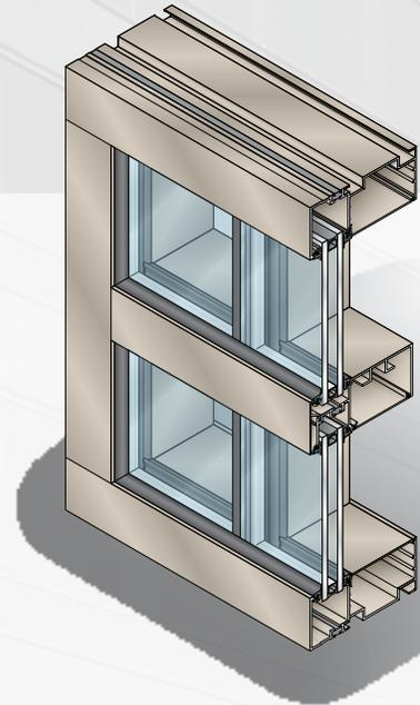
Our Butt Glazed Systems are vertically butt glazed horizontal ribbon window systems that are ideal for low to mid-rise applications. The BG and BT Systems are engineered for continuous long runs of glass creating a monolithic appearance. Intermediate horizontals can be added for accenting horizontal bands. The BT Series features the Poly-Aluminizer™ and Struct-Link™ Thermal Break Technology. These systems can be glazed from the interior or exterior.
