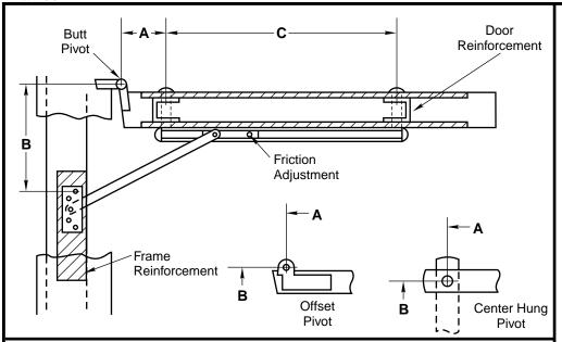
5. Install channel on door with "A" dimension sex bolt. Locate "C" dimension sex bolt hole making sure that channel is horizontal and parallel with stop strip. Drill 5/16 (7.9) dia. sex bolt hole and finish installing holder.
