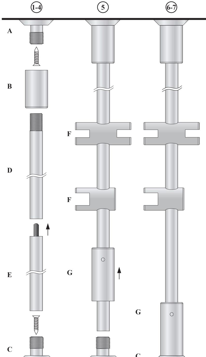
Top to Bottom - 10mm Rod installation
