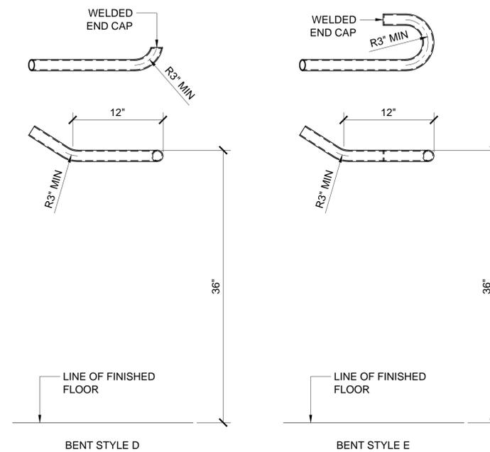
STANDARD WALL RETURN CONFIGURATIONS WITH BENT CORNERS
