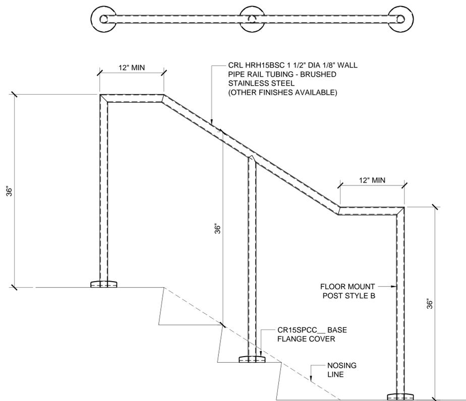
TYPICAL FREE STANDING HANDRAIL WITH MITERED CORNERS
