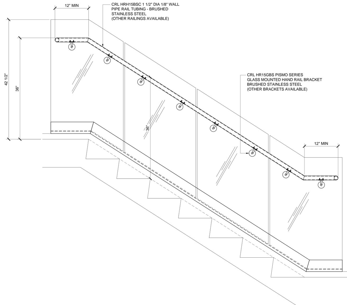
TYPICAL BENT GLASS-MOUNTED HANDRAIL
