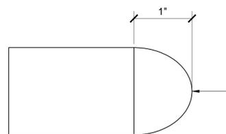
CRL WRDC15 WOOD DOME END CAP FOR 1 1/2" O.D. WOOD HAND RAILS
