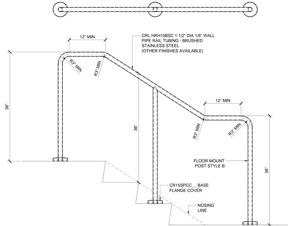
TYPICAL FREE STANDING HANDRAIL WITH BENT CORNERS
