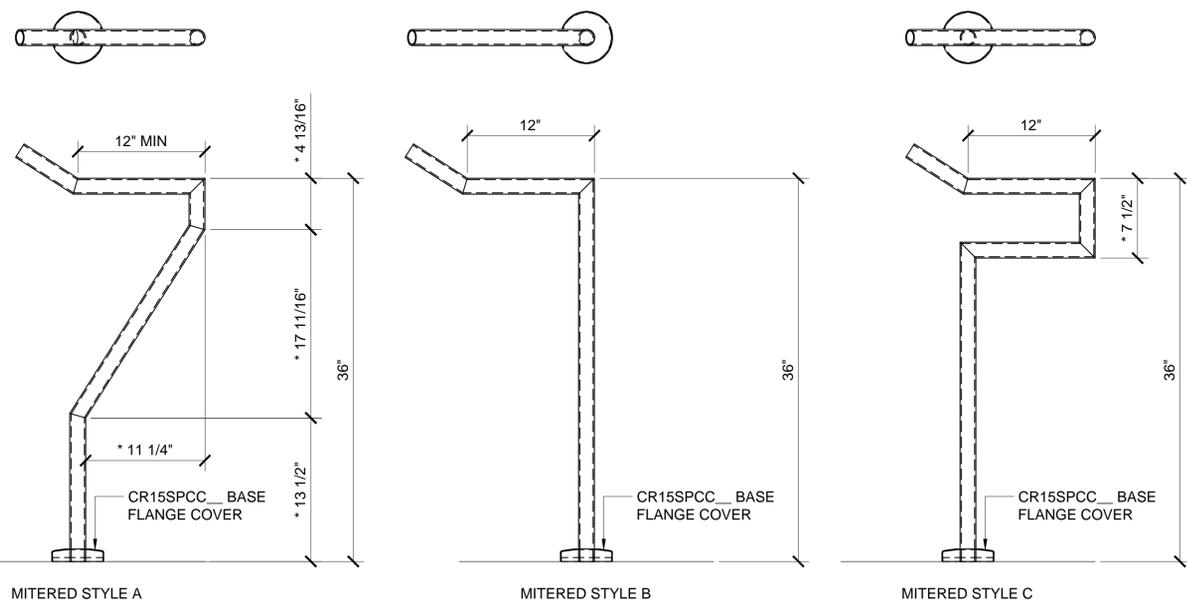
STANDARD FLOOR MOUNT CONFIGURATIONS WITH MITERED CORNERS
