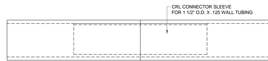
CRL CONNECTOR SLEEVE FOR 1 1/2" O.D. X .125 WALL TUBING
