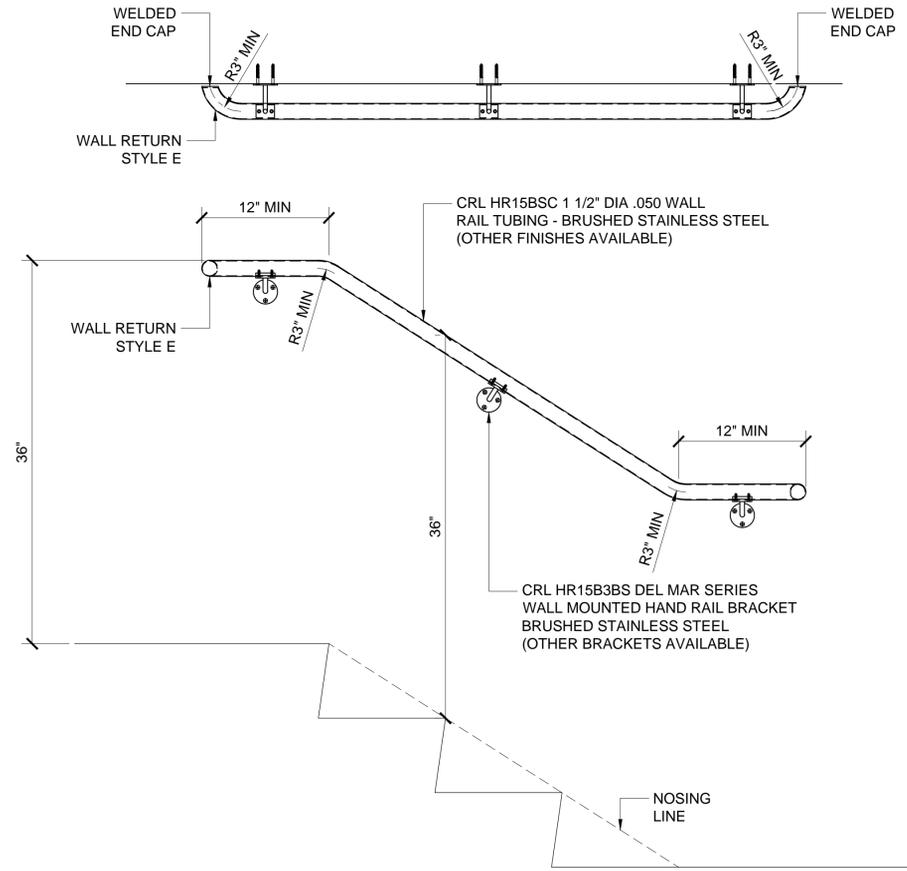
TYPICAL WALL-MOUNTED HANDRAIL WITH BENT CORNERS
