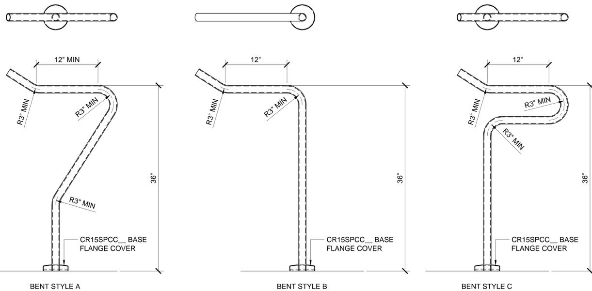
STANDARD FLOOR MOUNT CONFIGURATIONS WITH BENT CORNERS
