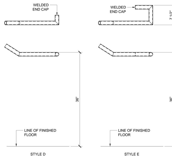
STANDARD WALL RETURN CONFIGURATIONS WITH MITERED CORNERS
