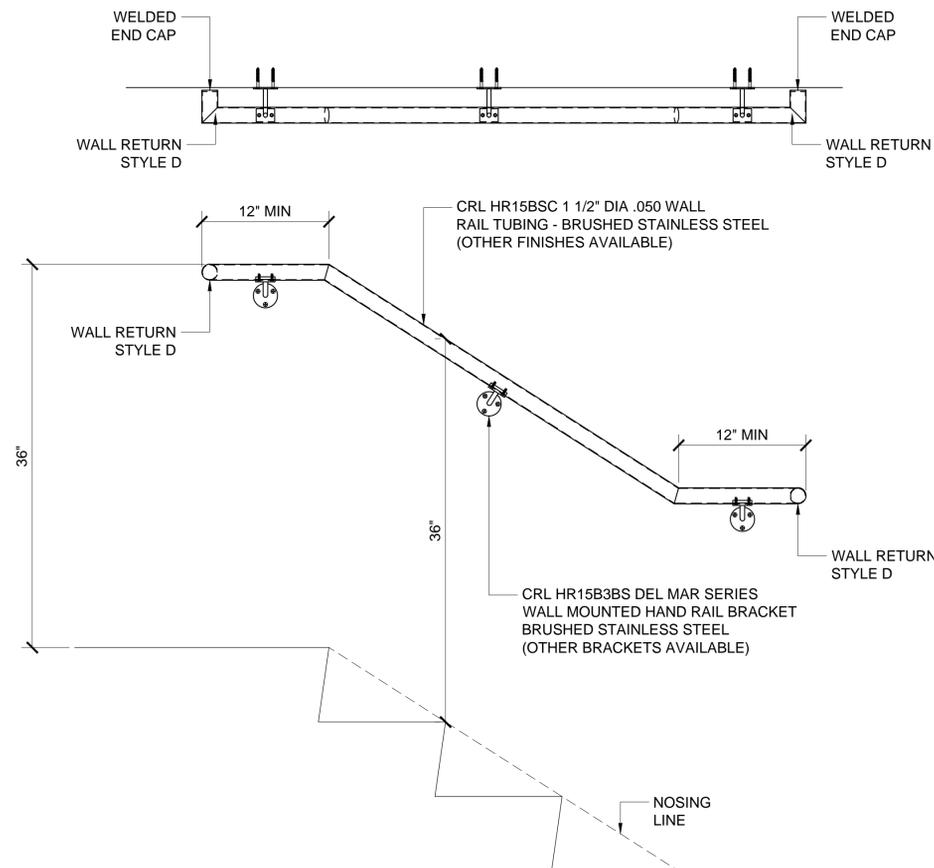
TYPICAL WALL-MOUNTED HANDRAIL WITH MITERED CORNERS
