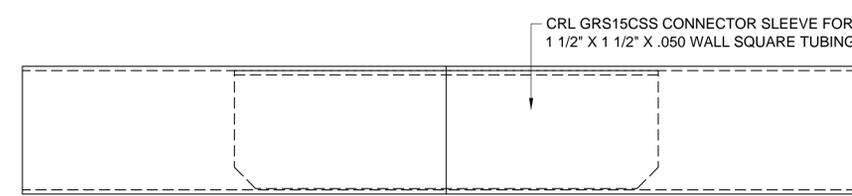
CRL GRS15CSS CONNECTOR SLEEVE FOR 1 1/2" X 1 1/2" X .050 WALL SQUARE TUBING
