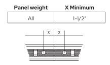
Track connectors are mandatory for all adjoined tracks in order to provide a continuous weight bearing surface.
