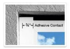
6. A final bead of caulking is recommended to achieve a permanent seal between the trim and the drywall.
