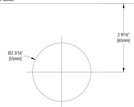
NOTE: The above template is for Top Mounted Locks. For bottom mounting rotate the template 180°. For side mounting rotate 90° either right or left. Centerline the lovk opposite the Keeper.
