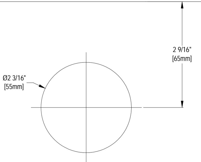
NOTE: The above template is for Top Mounted Locks. For bottom mounting rotate the template 180°. For side mounting rotate 90° either right or left. Centerline the lock opposite the Keeper.
