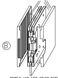
REMOVE VHB TAPE COVER PAPER APPLY COVER PLATES PRESS FIRMLY TO ENSURE ADHESION
