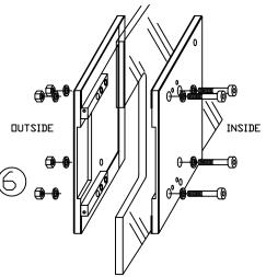
ASSEMBLE CLAMP PLATES ONTO GLASS. BE SURE TO HAVE NUTS AND WASHERS ON THE OUTSIDE
