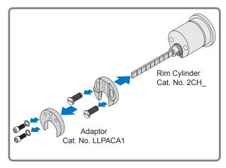
4. Disassemble new Rim Cylinder to rotate Flat Shaft to vertical position and reassemble.
