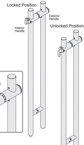
Loosen the two Mounting Post Set Screws and then remove the Interior Handle Screw at Lock Housing.
