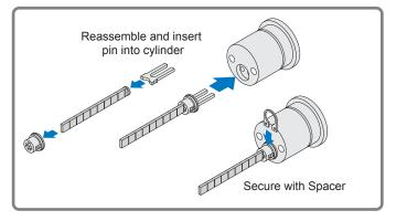
5. Install Adaptor on new Rim Cylinder and reattach to Exterior Handle.
