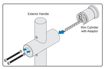
NOTE: Cat. No. 2CH\_ Rim Cylinder may be substituted with Rim Cylinders with vertical tail pieces at least 2-1/2" (64 mm) long.
