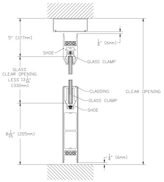
4" TAPERED DOOR RAIL TOP NON CLAD 10" SQUARE DOOR RAIL BOTTOM CLAD WITH NON CLAD HEADER
