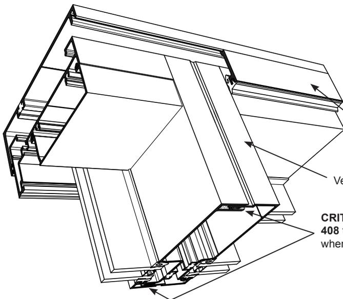
Apply **CRL RTV 408** Sealant between all vertical expansion joints **BEFORE** attaching the RW622 Compensation Channel Stop. Additionally, all connection joints of vertical members that will be covered by the RW622 should be filled with sealant. This includes jambs, mullions, splayed verticals and SG joints.
