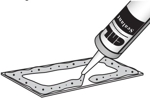
Run a 3" tall bead of silicone above the Subsill for 12 pounds (test pressure) of water.
