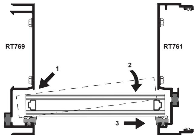
Install glass panel into frame by first angling the panel into the deep pocket. Swing the other end around and into the shallow pocket. Lower the panel down onto the setting blocks.
