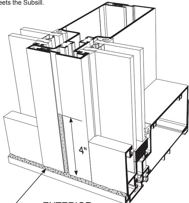
**CRITICAL SEAL:** Use **CRL RTV 408** to seal along the exterior Subsill and into gaps between Vertical Mullions.
