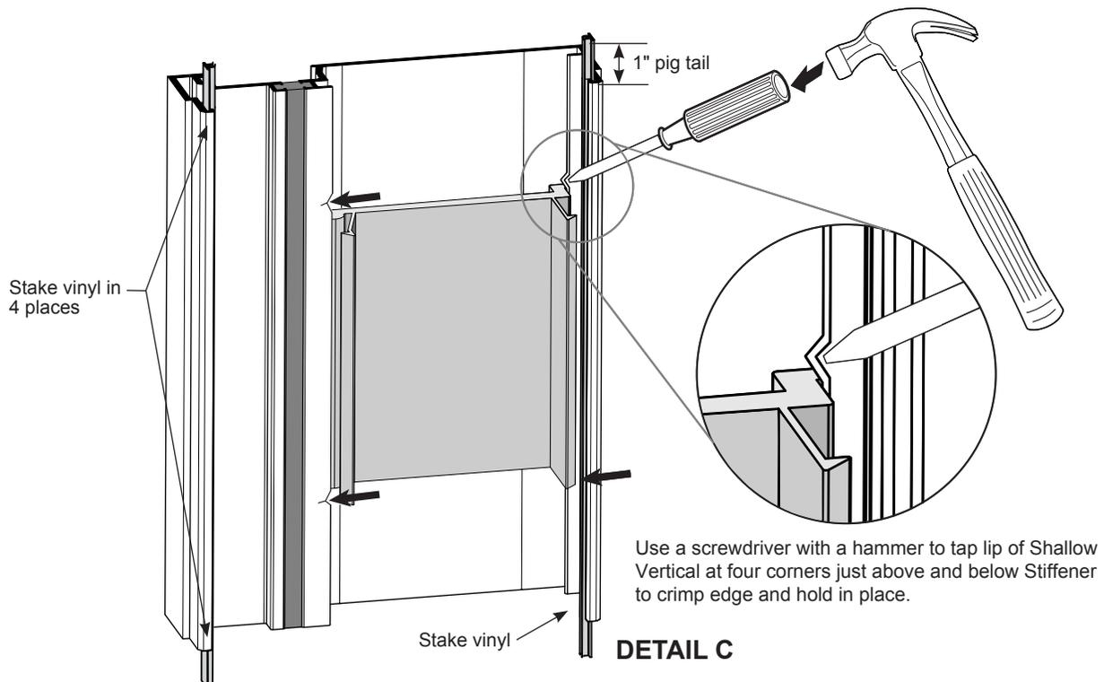
5. Slide in the VS200 vinyl into the RT761 mullion and leave a 1" pig tail at each end and stake in place.
