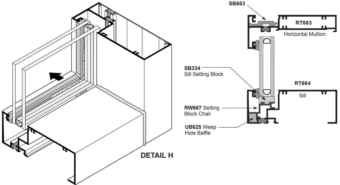
13. Push in temporary short wedges of the **NP606** Gasket to hold glass in place.
