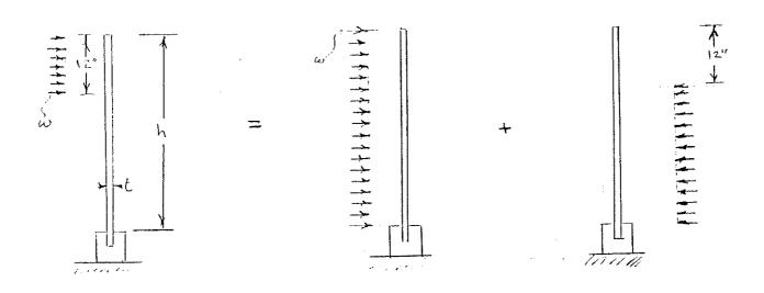
BOCA '96 specified loads per section 4.4 of ASCE7 (1995) "Minimum Design Loads for Buildings and Other Structures" Section 4.4.2A) requires that glass fillers must withstand 50# applied horizontally on an area not to exceed 1 ft.2. Normally, this load will be distributed over a large panel. For conservatism, it will be assumed that this load is applied on a 1 ft. wide panel, applied at the top to maximize bending stress.
