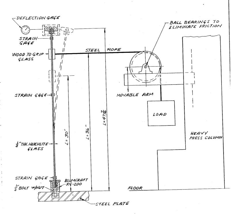
LOAD TEST EQUIPMENT FOR RAILGLASS
