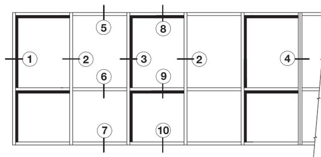
**NOTE:** NP225 E.P.D.M. Glazing Gaskets used on both sides of 1/4" (6) glass throughout. NP238 E.P.D.M. Glazing Gaskets for 3/8" (10) glazing.
