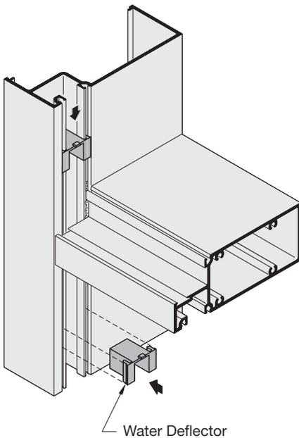
Apply silicone to two sides of glazing pocket at vertical/horizontal joint and glazing reglets. Slide water deflector, down into position. Seal over top edges of water deflector, leaving a gap on outside edge allowing water to drain into subsill.
