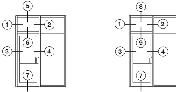
**NOTE:** NP225 E.P.D.M. Glazing Gaskets used on both sides of 1/4" (6) glass throughout. NP238 E.P.D.M. Glazing Gaskets for 3/8" (10) glazing.
