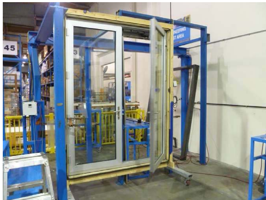
Photo No. 2 Door Cycling Set-up - Interior
