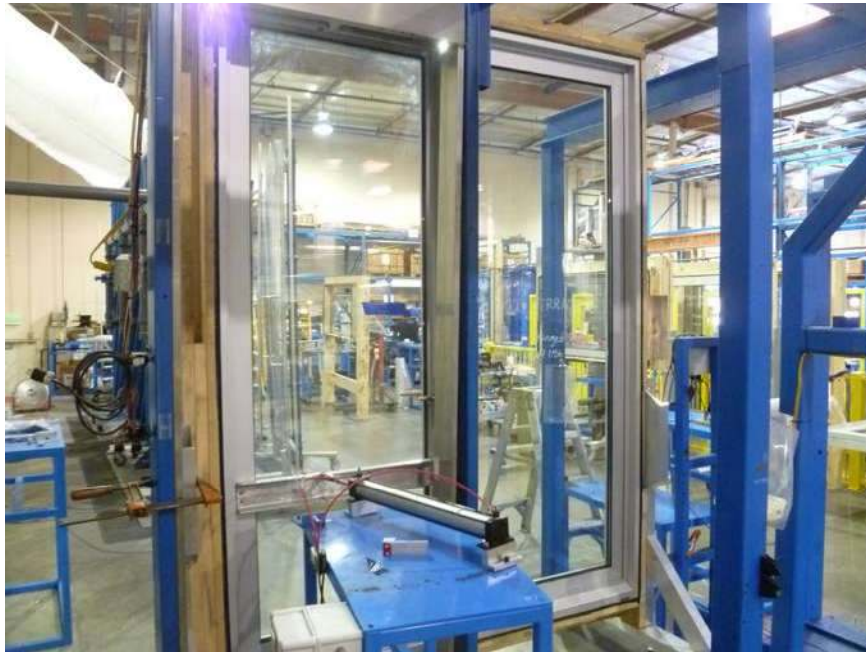
Photo No. 1 Door Cycling Set-up – Exterior
