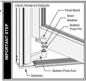
NOTE: A Shim Washer **MUST ALWAYS** be used on the Bottom Pivot Pin. Door failure may result without it. The spacing between the Pivot Block and the Pivot Arm is 3/32"-1/8" (2-3 mm).
