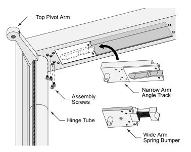
NOTE: it is advisable to use a #3 Phillips driver when attaching the four small screws provided. A screwgun with a #5 torque setting should be used if possible.
