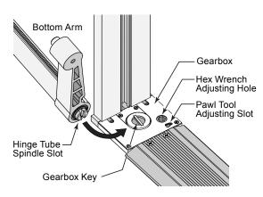
NOTE: Hinge Tube Spindle Slot must line up with Gearbox Key upon installation. Key can be rotated to align with Spindle Slot with 1/2" (13 mm) Hex Wrench (Not provided).
