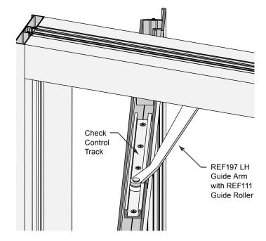
7. Attach the Guide Arm and Hub to the Check Spindle once again by opening or closing the door until the oval slots align. Secure arm with the 1/4"-20 X 1" FHMS using Cat. No. 24221 Loctite® 242® Threadlocker.
