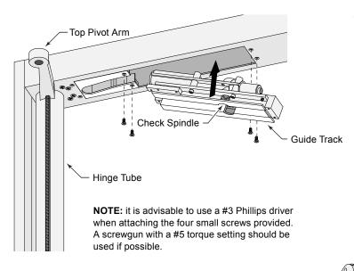
1. Install Guide Track Assembly with four short screws provided. Insert the assembly up into the head at an angle and drop back down onto the fastener holes.
