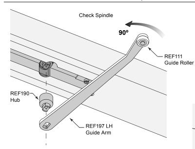
5. Place the REF190 Hub and REF197 LH Guide Arm onto the Check Spindle, align and hold in place with your hand. Using the Guide Arm, turn the Spindle until it is 90 degrees with the head. Remove the Guide Arm and Hub before continuing to the next step.
