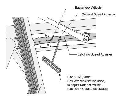
NOTE: Adjusting the screws too far open (CCW) can result in oil leakage.
