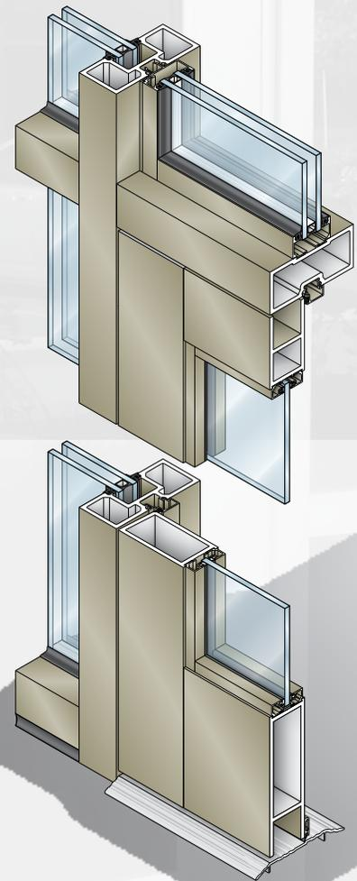
Durafront Doors and Frames are fabricated from tubular aluminum extrusions with a wall thickness of 3/16" (4.8 mm). These extra strong, long-lasting entrance packages are ideal for locations subjected to extremely high traffic flow. Durafront Entrance Packages are offered for center and offset hung doors. Offset hung doors are supplied with a pair and a half of heavy-duty hinges, pivot sets, or a continuous gear hinge. A variety of custom hardware is available upon request.
