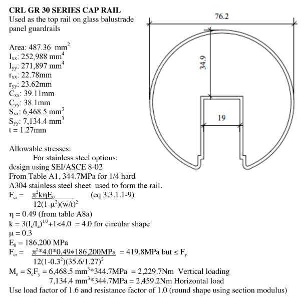
Determine allowable rail loads (ignoring deflection) for a maximum span of 1.5m Rail is continuous over multiple glass lights ( $M = wl^2/10$ )
