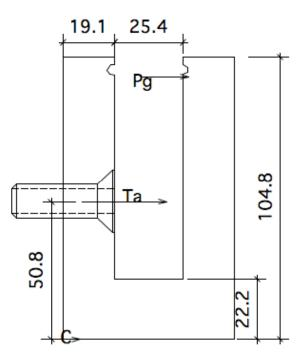
Screw or bolt strength = 39.2kN
