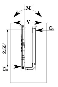
At maximum allowable moment determine bending in base shoe legs:  $M_s = C^*(0.188+2.55^{"}/2) + R_{C_B} *(0.188+2.55-0.425) =$  $M_s = 1,954^*(1.463) + 6,986 *(2.313) = 2.149$ kNm
