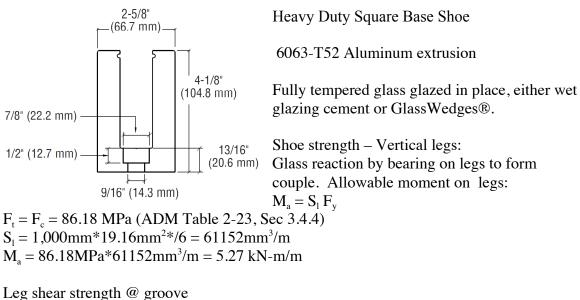
t<sub>min</sub> = 8.76mm  $F_v$  = 37.92MPa (ADM Table 2-24, Sec 3.4.20  $V_{all}$  = 8.76mm\*1000\*37.92MPa = 332.2 kN/m
