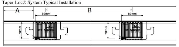
For 12mm Fully Tempered Glass and maximum glass height = 1,000mm (1100mm rail height):
