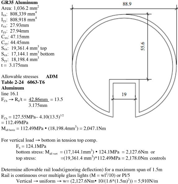
concentrated  $\rightarrow P = 2,127.6 \text{Nm} \times 5/(1.6 \times 1.5 \text{m}) = 4,432.5 \text{N}$
