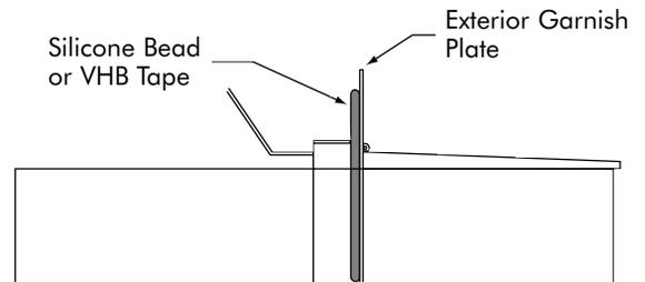
NOTE: If glazing panel is setting in a U-Channel, deduct the channel bottom thickness from the 3-7/8" measurement.
