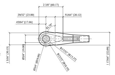
Tension strength of end at taper (minimum thread engagement depth)  $A = [(0.797/2)^2 - (0.472/2)^2]\pi = 0.324 \text{ in}^2$  End strength is greater than bar strength
