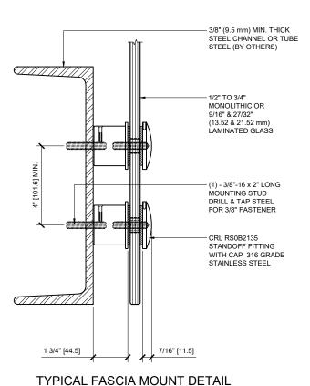
CRL RS0B2135 ON STEEL CHANNEL SUBSTRATE 6" =1'-0"
