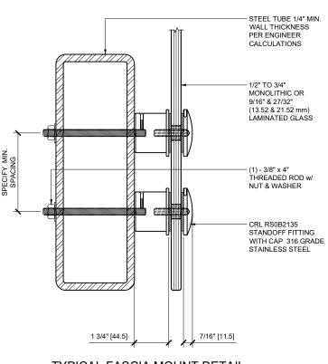
CRL RS0B2135 ON STEEL TUBE SUBSTRATE 6" =1'-0"
