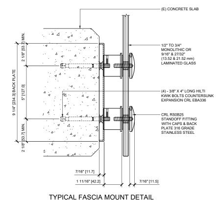
CRL RS0B25 ON CONCRETE SUBSTRATE 6" =1'-0"
