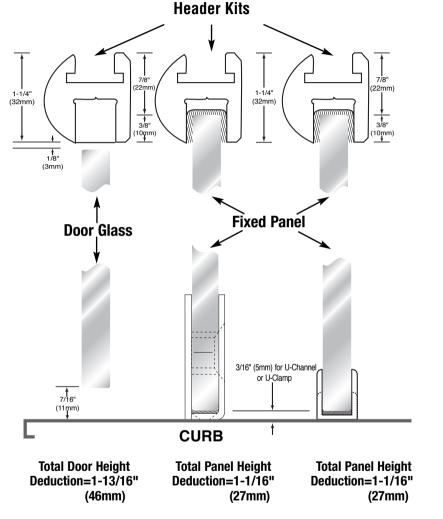
Example: You desire the top of the header to be at 80"(2032mm).
