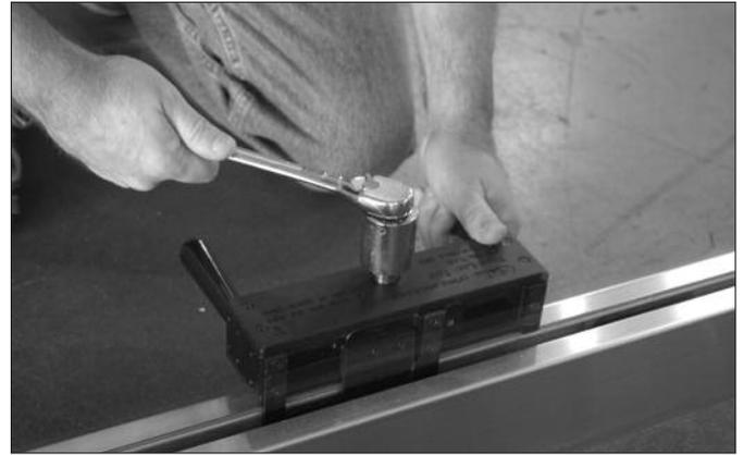
Make sure the blade movement mechanism of the TLK12 Tool moves freely, and hasn't become filled with dust or debris. Blade mechanisms that are poorly maintained may cause binding during the Taper compression operation, and result in an improper installation with insufficient compression of the Tapers.
