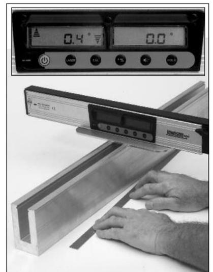
Use the "PAL" Tool to assure the Windscreen Base Shoe is level at all points. When leveling the Windscreen Base Shoe make sure you level the shoe within 0.4 degrees of the floor. Angular variation up to 0.4 degrees is acceptable during this process.
