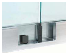
Step 2: Install glass panels with Setting/Centering Blocks and Sealing Pads between them to control the pour.
