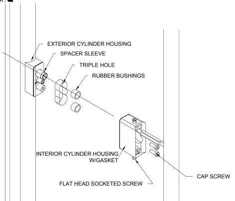
5. Back off locking nut and unwind the stud, being careful that the handle does not fall from the backside of the plywood. Remove rubber bushing for re-use during installation to the door.
