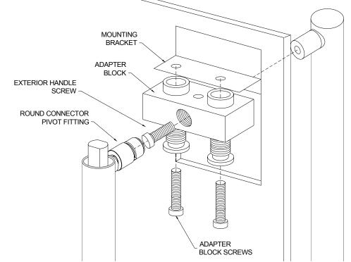
At the TOP Adapter Block, loosen up socket set screw and pull exterior handle away loose.
