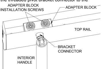
instructions for possible adjustments of the top rail. Wind the threaded pivot bracket connector to start thread.
