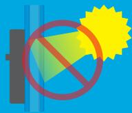
The Glass-Chek PRO uses a laser to measure the thickness of the glass and air space. The unit may be affected by *extremely* bright lights or facing the sun directly. The screen will display this error message if this condition occurs. Simply move to a different location, go to the other side of the window, or shade the laser aperture. If the window is operable you may be able open the window and reach through the opening to block the incident light from the back side of the meter.
