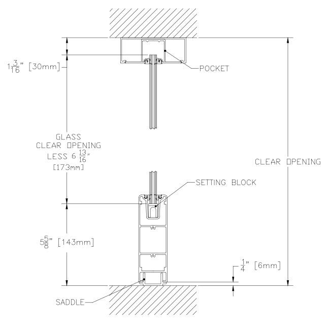
NON-CLAD HEADER WITH GLAZING POCKET TOP 6" SQUARE SIDELITE RAIL WITH 1/4" SADDLE AND SETTING BLOCK BOTTOM NON-CLAD
