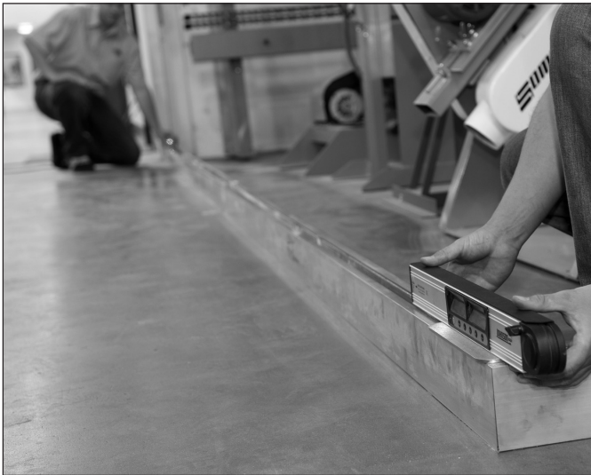
Align the "PAL" Digital Laser Tool Cat. No. 406065 with Base Shoe and point toward the Laser Target set at other end of Base Shoe.
