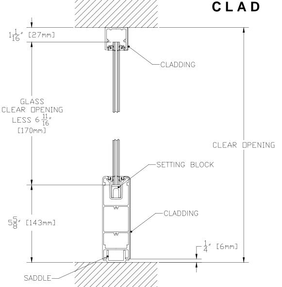
U-CHANNEL TOP 6" SQUARE SIDELITE RAIL WITH 1/4" SADDLE AND SETTING BLOCK BOTTOM CLAD OR NON-CLAD
