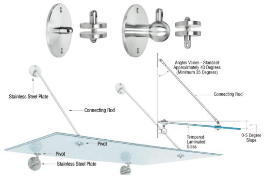
Support hardware for flat panel awnings such as laminated glass. (GAS90 shown above)
