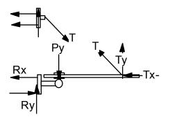
Reaction from connecting rod:  $T = V/(Sin\alpha)$  (Rod tension or compression)  $\alpha = rod$  angle 35° min to 55° max, typically rod length is sized for  $\alpha = \pm 45^{\circ}$ Horizontal load -  $H = V/(Tan\alpha)$ For wind uplift bar will act in compression.  $1.22V \le T \le 1.74V$
