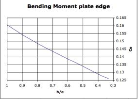
For 3' awning width with PVB interlayer  $S = 2*0.377^2 = 0.284 \text{ in}^3$ Allowable bending moment on glass is: Wind:  $M_{al} = 9,600 \text{ psi}*0.284 \text{ in}^3/\text{ft} = 2,726''#/\text{ft} = 227.2'#$ Live:  $M_{al} = 4,550 \text{ psi}*0.284 \text{ in}^3/\text{ft} = 1,292''#/\text{ft} = 107.68'#$ Snow:  $M_{al} = 4,550 \text{ psi}*0.284 \text{ in}^3/\text{ft} = 1,292''#/\text{ft} = 107.68'#$ Dead:  $M_{al} = 3,300 \text{ psi}*0.284 \text{ in}^3/\text{ft} = 937''#/\text{ft} = 78.1'#$
