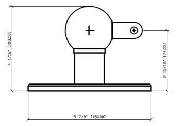
Maximum load on rod for 35° angle: Controlled by glass bracket.  $H \le 1,245\#$   $Y \le 1,245*Tan35^\circ = 872\#$   $T \le \sqrt{(1,245^2+872^2)} = 1,520\#$ Maximum load on rod for 45° angle:  $H \le 1,245\#$   $Y \le 1,245*Tan45^\circ = 1,245\#$   $T \le \sqrt{(1,245^2+1,245^2)} = 1,761\#$ Maximum load on rod for 55° angle: Controlled by wall bracket.  $Y \le 1,600\#$   $H \le 1,600*Tan35^\circ = 1,120\#$  $T \le \sqrt{(1,600^2+1,120^2)} = 1,953\#$
