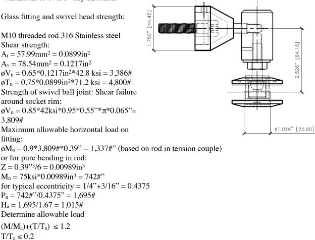
Check connection rod between standoff fitting body and wall mount:  $A_t = 0.1495 \text{ in}^2$   $A_v = 0.196 \text{ in}^2$   $V_a = 0.55*75 \text{ksi}*0.1495 \text{in}^2/2= 3,083 \#$   $T_a = 0.1495 \text{in}^{2*}75 \text{ ksi}/2 = 5,606 \#$   $Z = 0.5^3/6 = 0.02083 \text{ in}^3$  $M_a = 0.02083*75 \text{ ksi}/1.67 = 936" \#$
