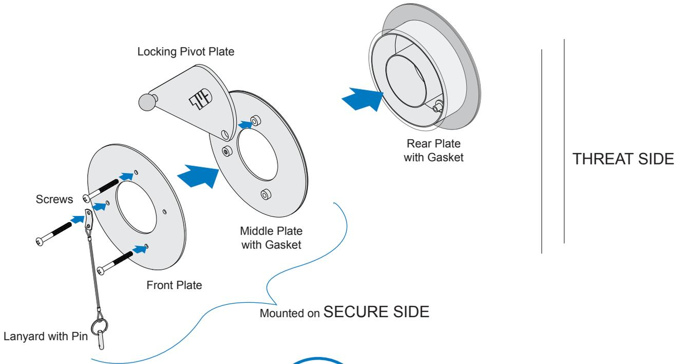
Swing Locking Pivot Plate closed and insert Pin to lock.
