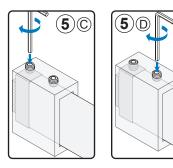
NOTE: Ensure Header is level. If not, loosen screws holding Mounting Blocks to adjust height.
