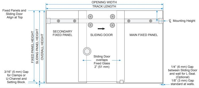
NOTE: Drawings not shown to scale. Track is cut 1" (25 mm) less than Opening Width and centered in opening. Overall Height is height from curb/floor to top of glass. Drawings shown from interior with Bottom Door Guide cupping Fixed panel. See Page 8 for Guide mounting options.
