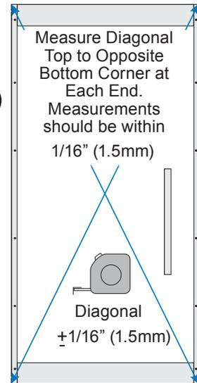
2. Loosen the set screws on both sides of the Lead Stile with included Hex Driver. Use Phillips Screwdriver to turn Adjuster Screw. Check measurements again. If the door is square, tighten the set screws and move on to installation. If not, go to Step 3 below.
