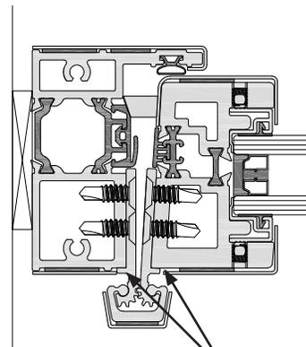
Gear Hinge must be Flush with Door & Frame
