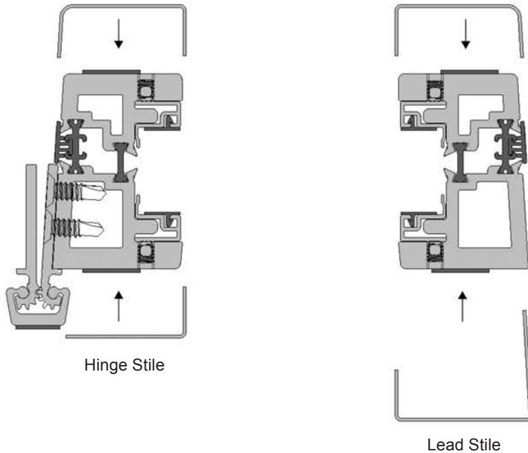
2. Remove liner from VHB Tape and apply Clad to Gear Hinge, make sure to wipe clean cladding using solvent before installing
