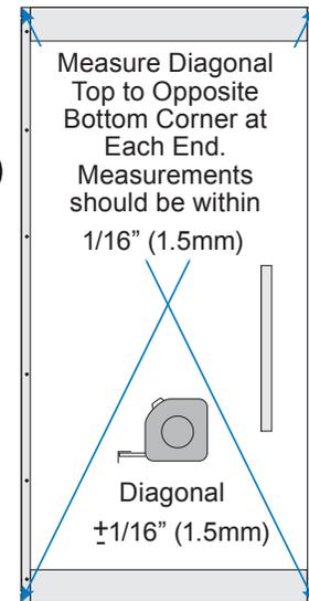
3. Loosen set screws on both sides of Lead and Pivot Stiles. Use Phillips Screwdriver to turn Adjuster Screw. Make sure glass fully rests on bottom setting block. Check measurements. When the door is square, tighten all set screws and move on to installation.
