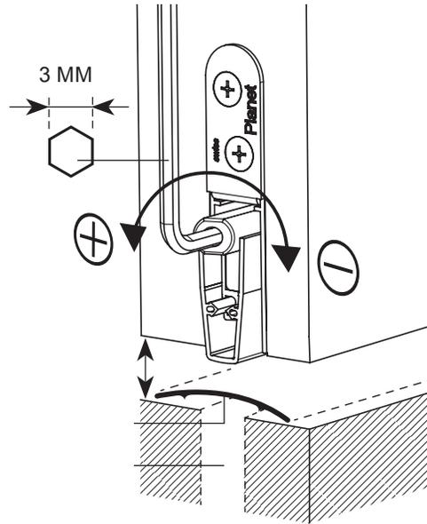
2. Please note the orientation of the beveled actuator below. Actuator contact with frame jamb will engage drop seal.
