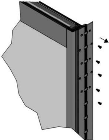
2. For hinge side of Frame Jamb, please use the provided gear hinge as a template to prep for #12 pilot holes. Make sure Gear Hinge is installed per dimension shown in image below
