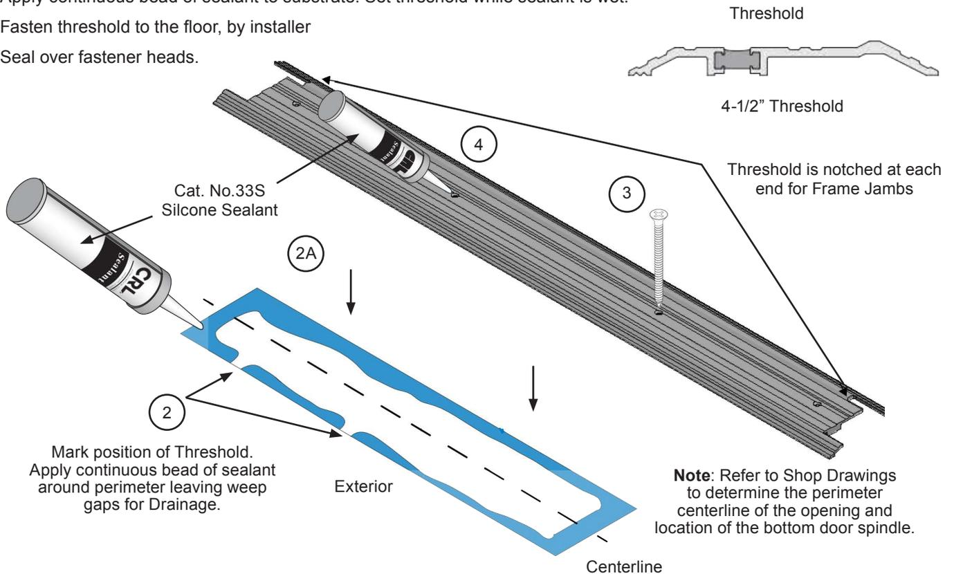
5. Align Threshold to Up & Over Frame
