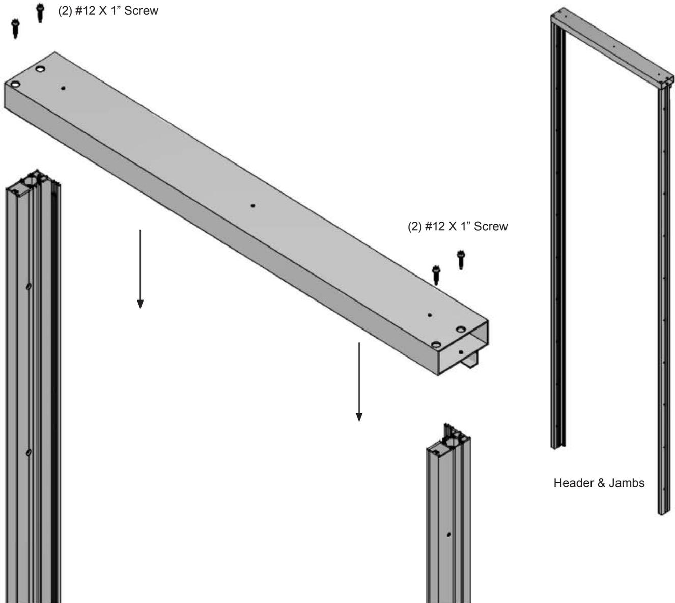
2. Once Header is securely fastened to Jambs (Hinge and/or Lead) proceed to installing up & over frame into rough opening.
