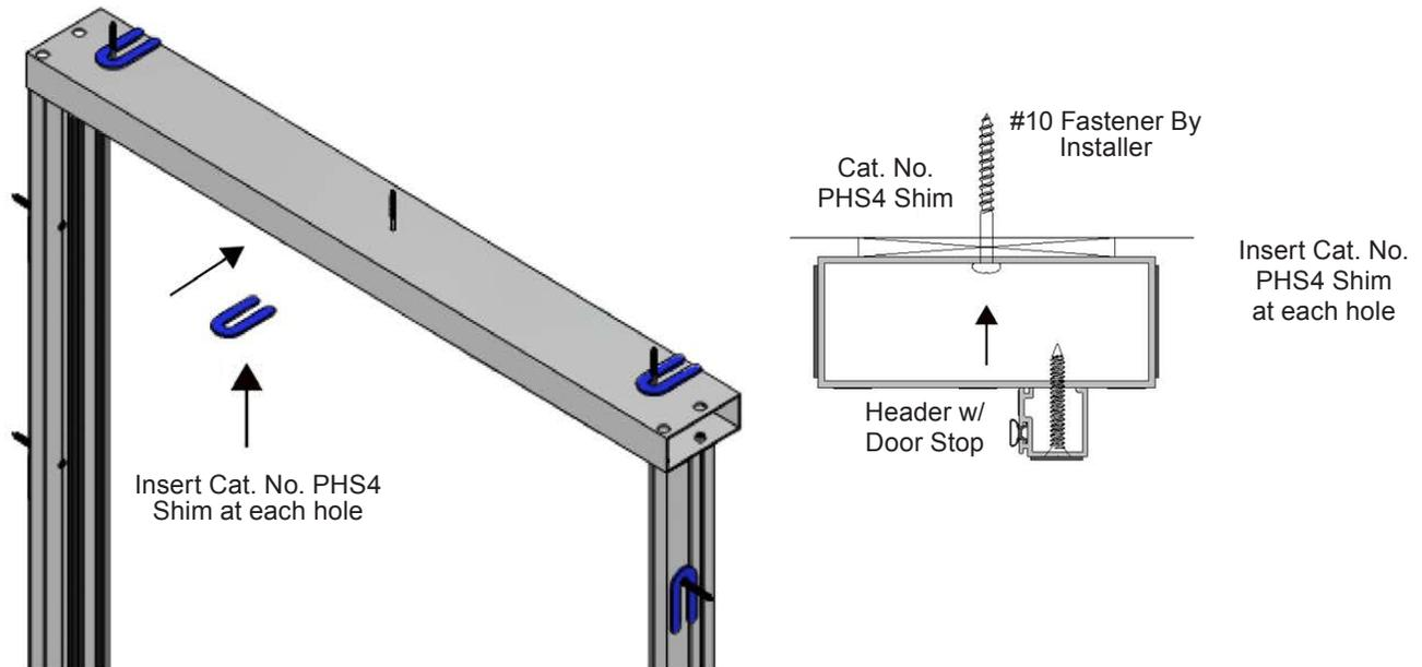
2. Once Shims are installed/placed, proceed with fully fastening Header & Frame Screws into place
