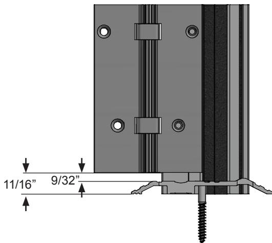
2A. Please make sure Gear Hinge butts up flush with Door & Frame
