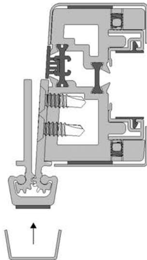
**Note:** Door Rail Clad will be pre-installed by CRL
