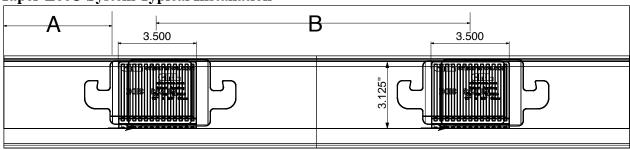
**Taper-Loc® System Typical Installation**
