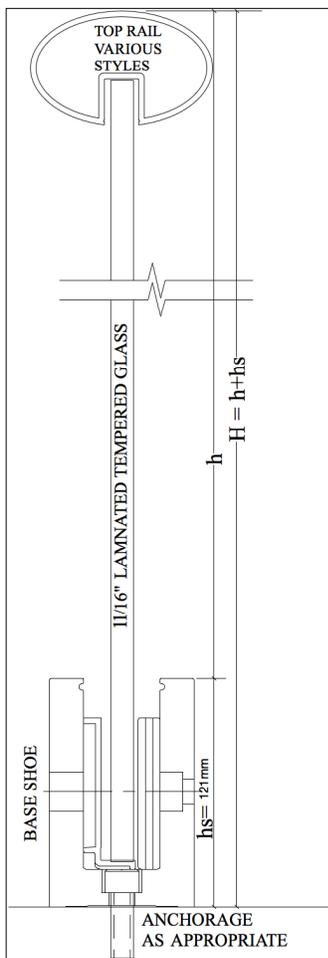
FOR WIND SCREEN OR DIVIDER APPLICATIONS WHERE FALL PROTECTION IS NOT REQUIRED THE CAP RAIL MAY BE OMITTED.
