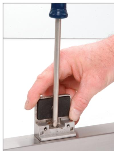
Lastly, insert the screw or bolt into the Rivet-Nut and tighten
