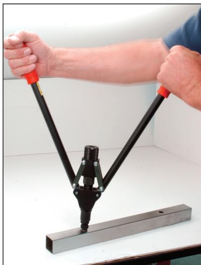
Third, compress the Rivet-Nut by using the CRL Cat. No. 34604 Heavy-Duty Thread Insert Tool (FIG. 2)
