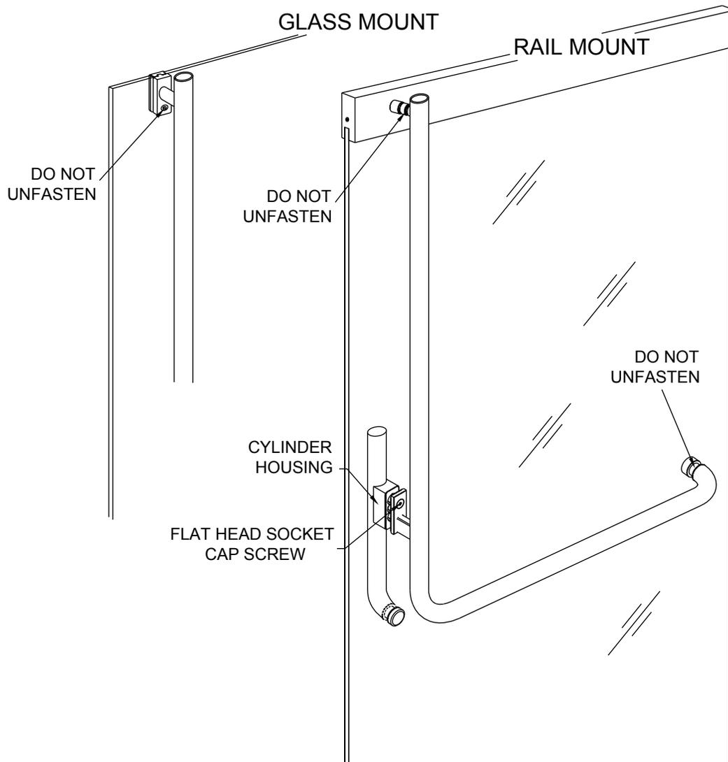
1. Hold on to exterior cylinder housing.
