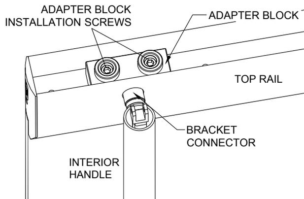
If experiencing difficulties aligning top pivot bracket connector with the hole on the rail, please refer to the
