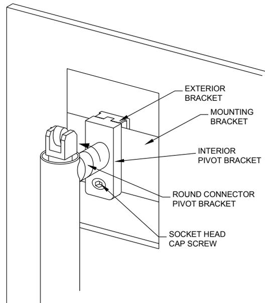
3. Remove threaded pin from bottom of horizontal handle and pull horizontal handle away from plywood. Use the CRL Spanner Wrench (part number MPHSW) to remove exterior cap retainer and rubber bushing. ➡
