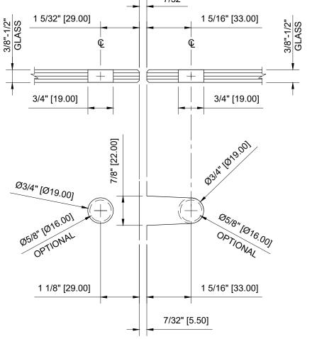
MOVABLE TRANSOM GLASS TO GLASS CLAMP 3/4" (19mm) DIAMETER HOLE 5/8" (16mm) DIAMETER HOLE (OPTIONAL) 7/32" (5.5mm) GLASS GAP GLASS FABRICATION TEMPLATE
