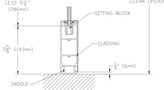
6" SQUARE SIDELITE RAIL WITH 1/4" SADDLE TOP 6" SQUARE SIDELITE RAIL WITH 1/4" SADDLE AND SETTING BLOCK BOTTOM CLAD OR NON-CLAD
