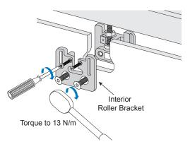
4. Place Glass Door on Wooden Shims to maintain 1/4" (6 mm) gap at bottom. Align notches in top of glass with Roller Brackets. Adjust height to fit.
