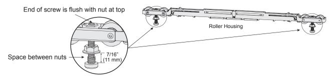
2. Loosen screws on metal plates on top of Dampeners so they can slide into grooves at top of Header Track.
