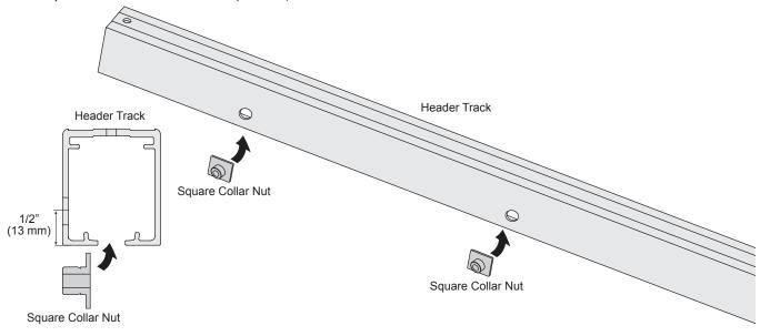
2. Fit white Plastic Collar over Square Nut from outside Header Track and snap into place.
