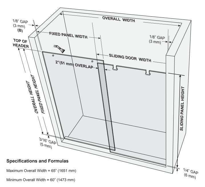
Metal Header Cut Length = Overall Width minus 5/8" (16 mm)
