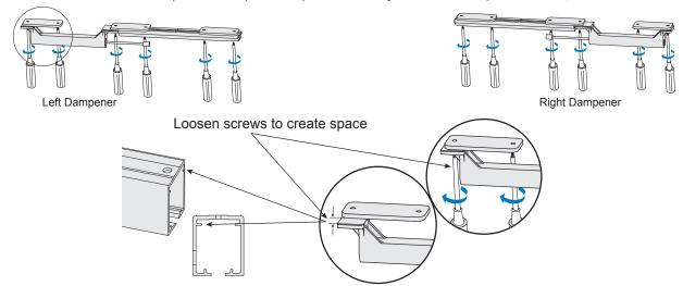
3. Slide Roller Housing into Header Track.
