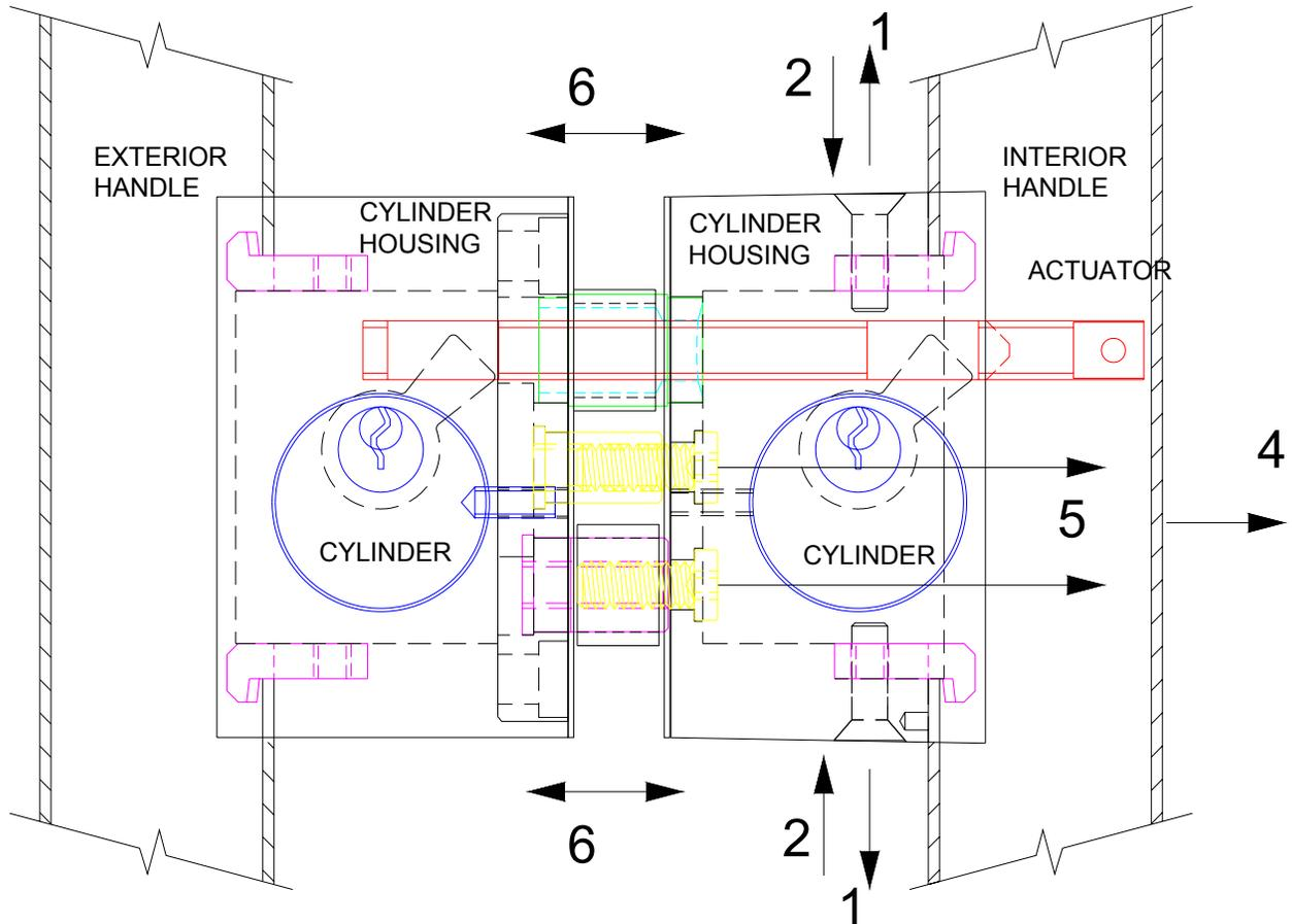
3. Remove the threaded pin from the bottom of the handle.
