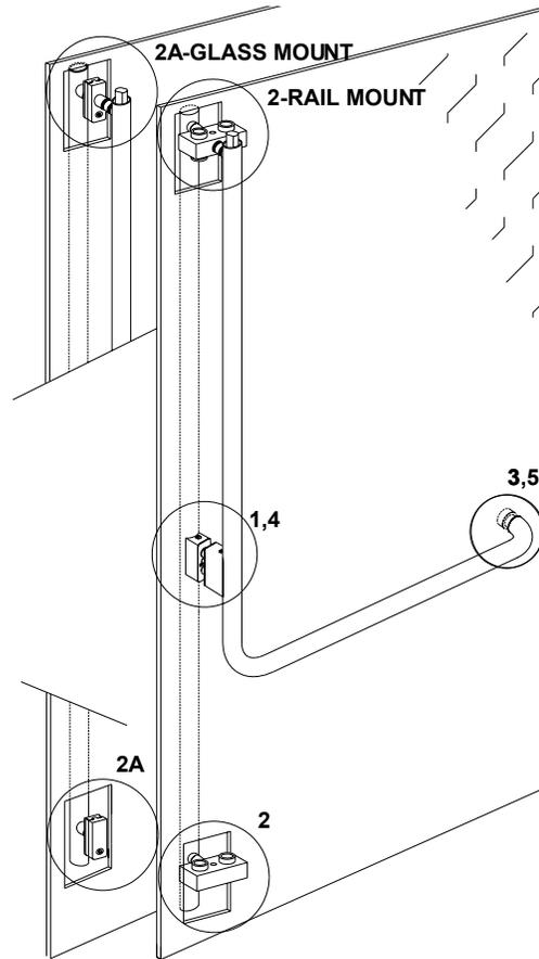
1. To remove the Handle from the board first loosen two flat head socket screws (A) so they protrude approximately 1/4" from Cylinder Housing (B) being careful NOT TO REMOVE them. Push or tap screws flush (C).
