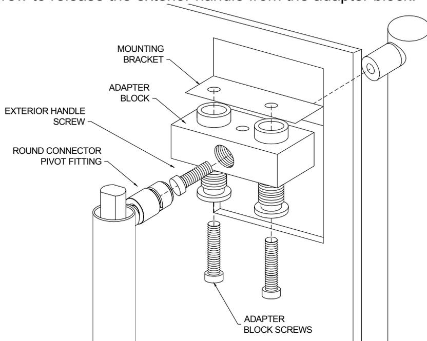
At the bottom Adapter Block, loosen up socket set screw and pull exterior handle away loose.
