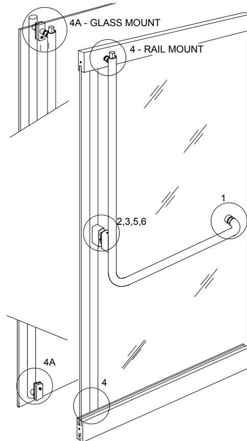
1. Insert rubber bushings into glass holes for exterior retainer cap. Place the retainer in position on exterior side of glass and tighten retainer cap through rubber bushing. Install stud with locking nut through washer w/gasket and tighten. ↓
