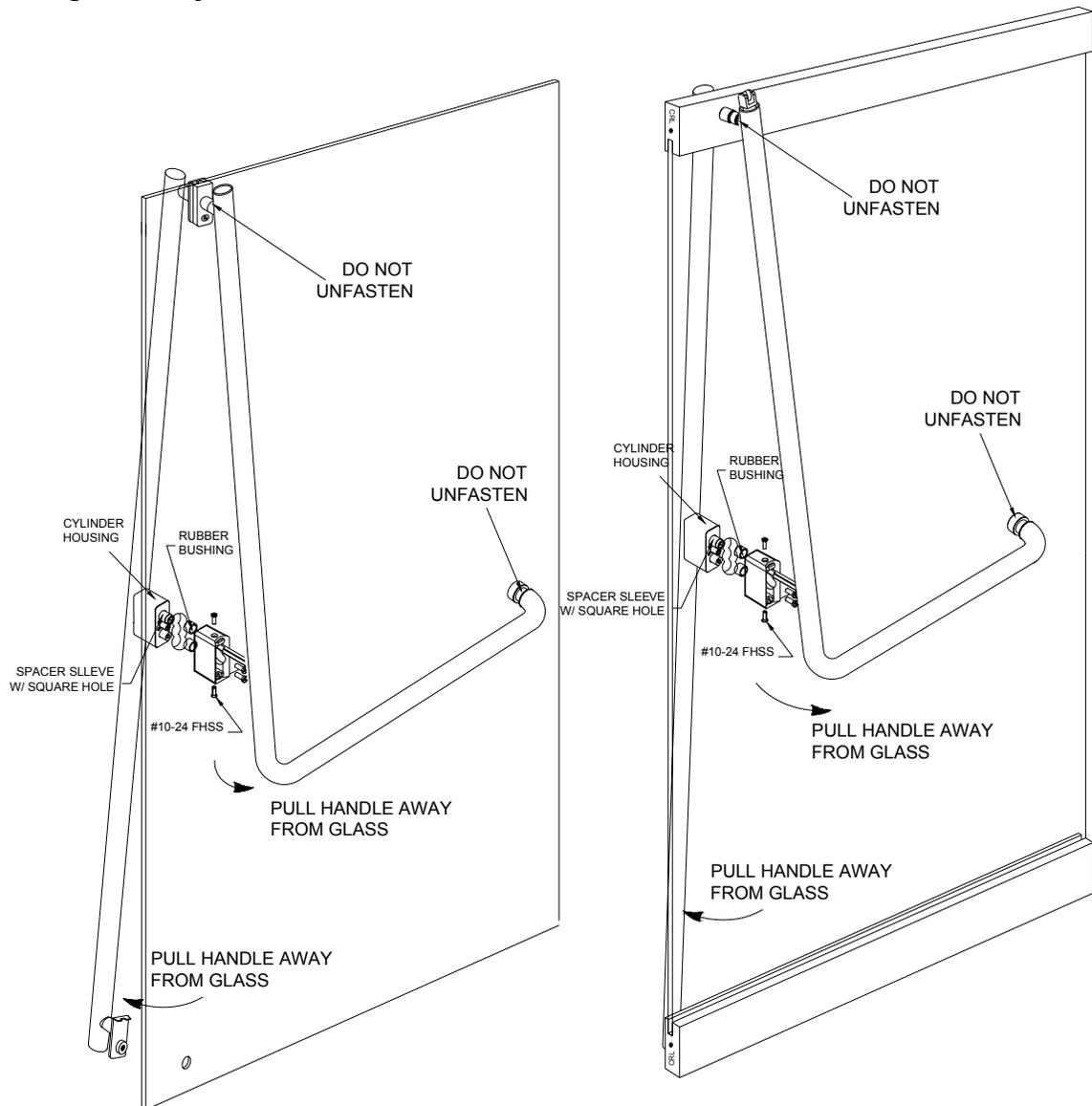
1. Loosen the flat head cap screws for approximately 1/8".
