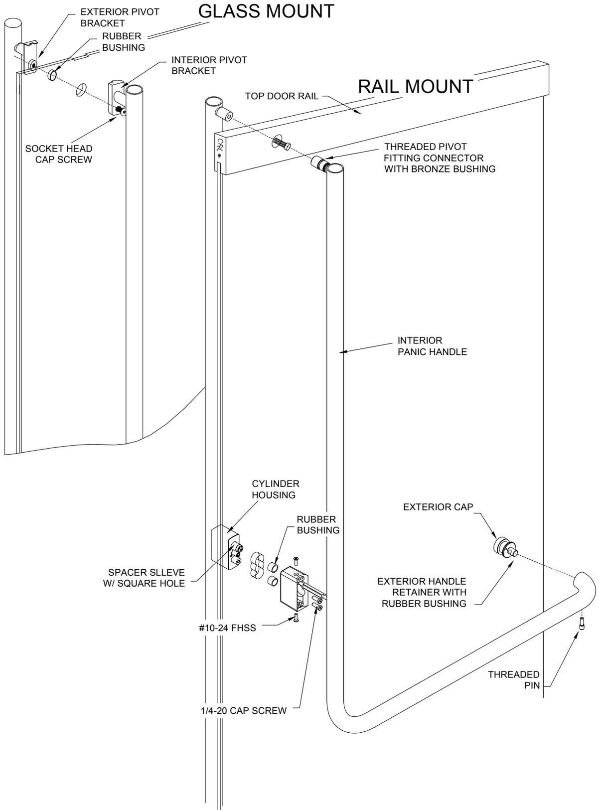
2. Install exterior lock housing with rubber bushing and spacer sleeve being careful that the square hole is facing the exterior handle with sides of hole in line with the handle width, and the lock cylinders in both housings are facing the hinge side of the doors. For installation of both housing together use two 1/4-20 cap screws. Finger tight.
