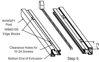
5. 3.5" Glass Edge Blocks installation: Peel adhesive back and place (2) edge blocks alongside glazing channels, 15" from each end.
