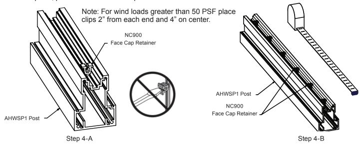
Align and insert snap clip's tabs into center channel. Turn clockwise ¼ to lock in place. DO NOT USE SCREWDRIVER TO INSTALL CLIPS. Pliers may be used to make the 1/4 turn.
