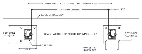
Note: Post to post spacing by engineering calculations. Max post spacing center to center is 5 feet.
