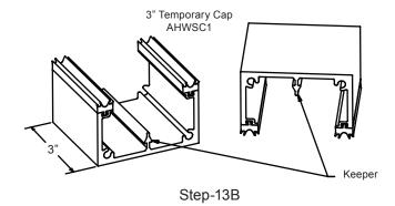
IMPORTANT – Temporarily hold glass in place with temporary cap at all four corners of glass. Align the keeper with plastic clips and push until cap locks in place. To remove temporary cap SLIDE CAP UP OR DOWN until it disengages from the plastic clip. Avoid pulling the cap horizontally. If clips are damaged in this process, replace with new ones.
