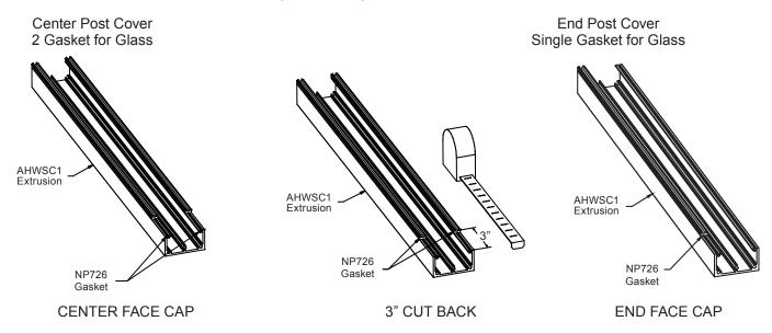
End Face Cap: Install gasket NP726 on the side of the post where glass will be installed only.
